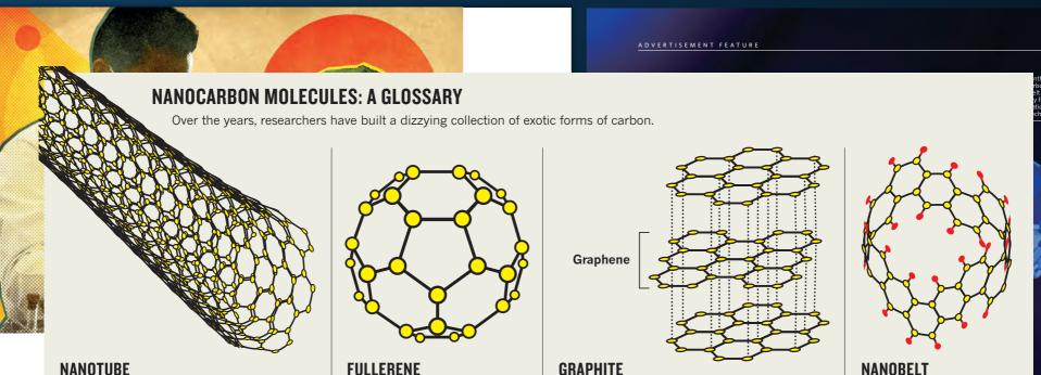
A sheet of hexagonally arranged carbon atoms, stretched to make a pipe shape. First formally described by scientists in 1952.
